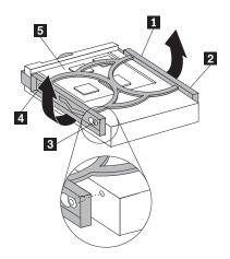
Figure 22. Installing the secondary hard disk drive into the bracket
